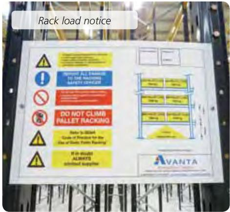
**Load notices** are supplied with all Avanta pallet racking installations in accordance with SEMA regulations.
