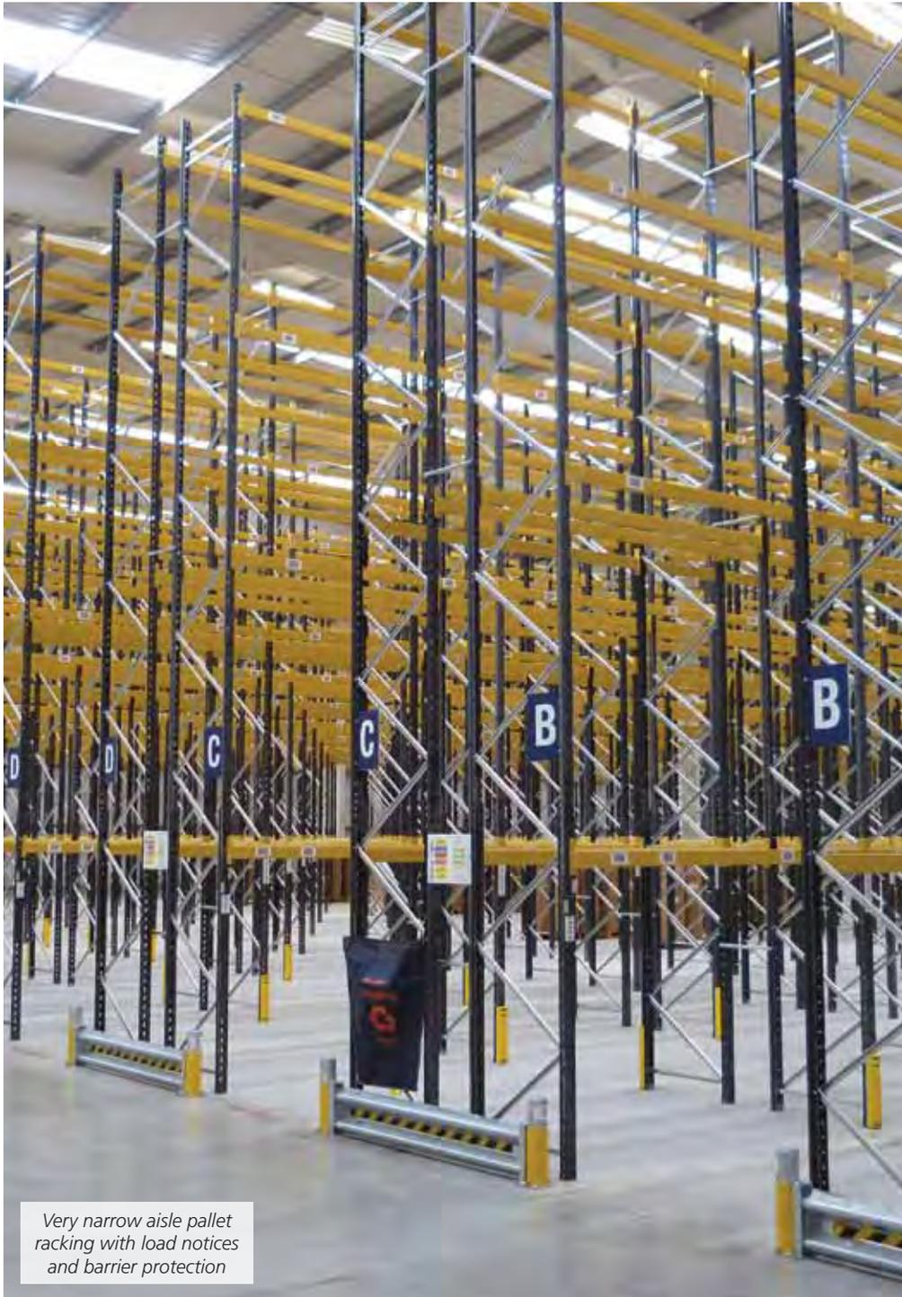
Very narrow aisle pallet racking with load notices and barrier protection
