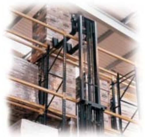
Lift trucks with telescopic forks are used to make efficient use of double-depth pallet racking.
